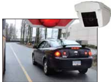
Camera 7 – 16 mm lens: exterior stop arm driver's side
