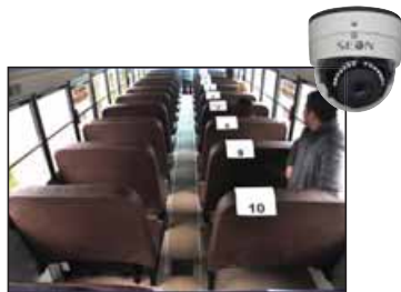
Camera 6 – 3.6 mm lens: up aisle rear to front
