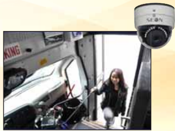
Camera 2 – 3.6 mm lens: driver/stairwell
