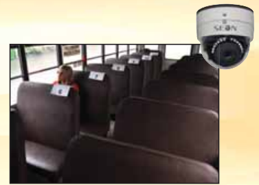
Camera 4 – 3.6 mm lens: 4th row down aisle
