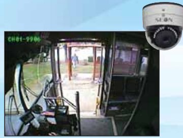
Camera 3 – 3.6 mm lens: driver/stairwell
