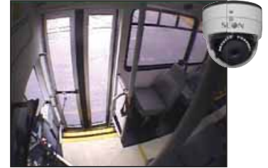
Camera 2 – 2.9 mm lens: driver/stairwell
