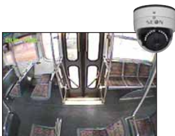
Camera 5 – 3.6 mm lens: exit door/stairwell
