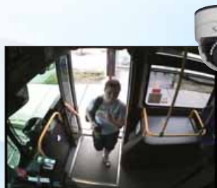
Camera 2 – 2.9 mm lens: driver/stairwell
